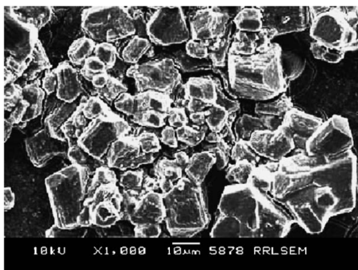
Scanning electron microscopic view of CLEC laccase Surface area ( \text{m}^2/\text{g} ) 2.456
