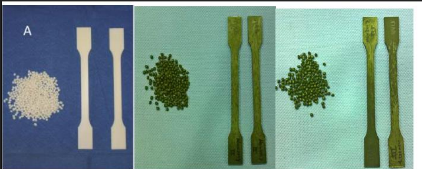
Figure 7. Examples of pellets and tensile bars of compound (A) N17-I (reference), (B) N17-II (C1201 + 25% Microalgae (MAB)) and (C) N17-III (C1201 + 25% Chlorella vulgaris ).
