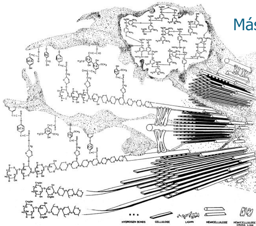
Figure 1. Secondary cell-wall (CW) structure. Components are arranged so that the cellulose microfibrils and hemicellulosic chains are embedded in lignin. Specific linkages and components of non-core lignin are shown for a generalized grass secondary CW. Non-core lignin components include p -coumaric (pCA), ferulic (FA), p -hydroxybenzoic (BA), sinapic (SA), and cinnamic (CA) acids.
