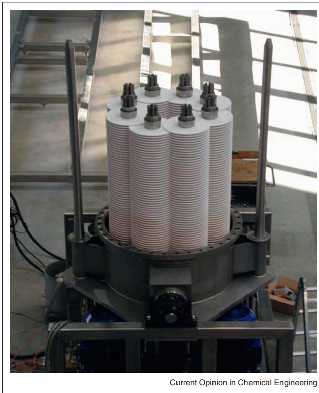
Industrial MSD module with 8 parallel shafts and 31 cm ceramic disks. Courtesy of Westfalia Separator.
