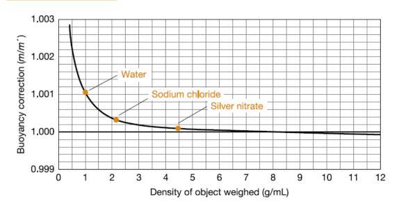
A pure compound called "tris" is used as a *primary standard* to measure concentrations of acids. The volume of acid required to react with a known mass of tris tells us the concentration of the acid. Find the true mass of tris (density = 1.33 g/mL) if the apparent mass weighed in air is 100.00 g.
