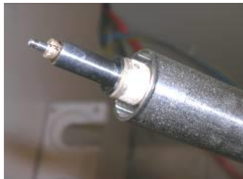
Heated by program, sample holding stick 200-300°C
