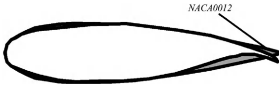
FIGURE 4.5 The NASA SC(2) 0712 supercritical airfoil overlaid on top of a symmetric NACA 0012 airfoil in the background.
