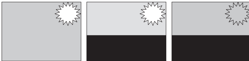
FIGURE 9.16 The environment measured by a green-sensitive sensor is illustrated on the left; in the center is the same measurement by the ultraviolet sensor. With the correct weighted sum of the two sensors, the effect of the sun can be removed.
