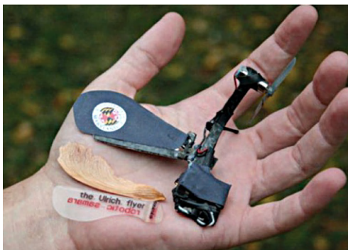
FIGURE 5.13 Mechanical samara microflyer, total mass 9.5 g, maximum dimension 75 mm [59]. Credits: E.R. Ulrich, D.J. Pines, J.S. Humbert, From Falling To Flying: The Path To Powered Flight Of A Robotic Samara Nano Air Vehicle, Bioinspiration & Biomimetics , 5, 045009, 2010.
