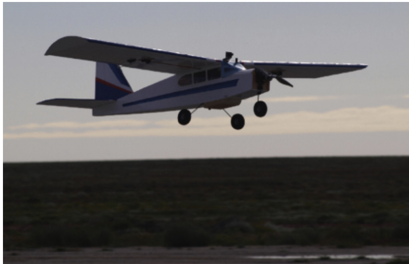
FIGURE 9.26 The UAV used for the flight trials was an electric-powered model aircraft with a 2m wingspan. It was fitted with an autopilot capable of conventional GPS/inertial flight and customized autonomous modes of flight. The optical-flow sensor was configured to gaze directly downward.
