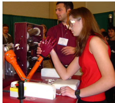
Figure 5. An EAP driven arm made by students from Virginia Tech and the human opponent, a 17 year old student.
