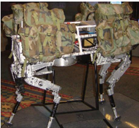
Fig. 11. The Big-Dog (made by Boston Dynamics), which is a mull-like legged robot that was developed for military application. Photographed by the author.
