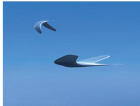
Fig. 9. A flying mechanism that mimics a bird was proposed for planetary exploration missions. Courtesy of Anthony Colozza, Ohio Aerospace Institute.
