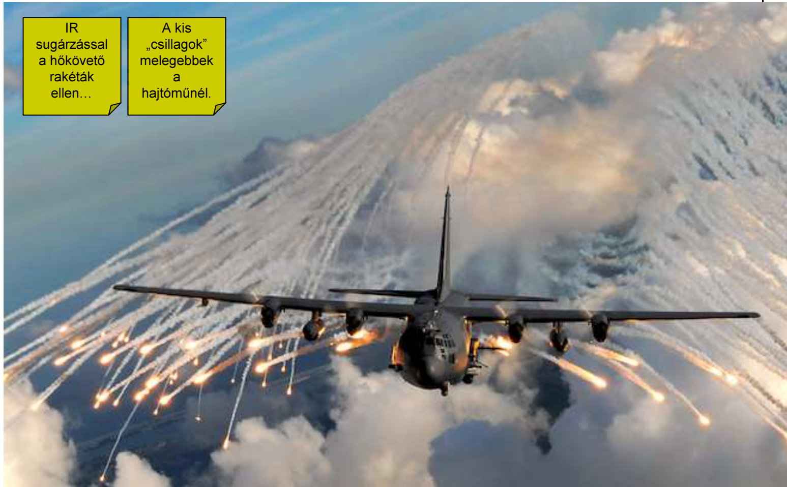
An AC-130U gunship fires flares to emit masses of infrared and confuse heat seeking missiles. http://www.wired.com/dangerroom/2012/10/infrared-obscurant/
